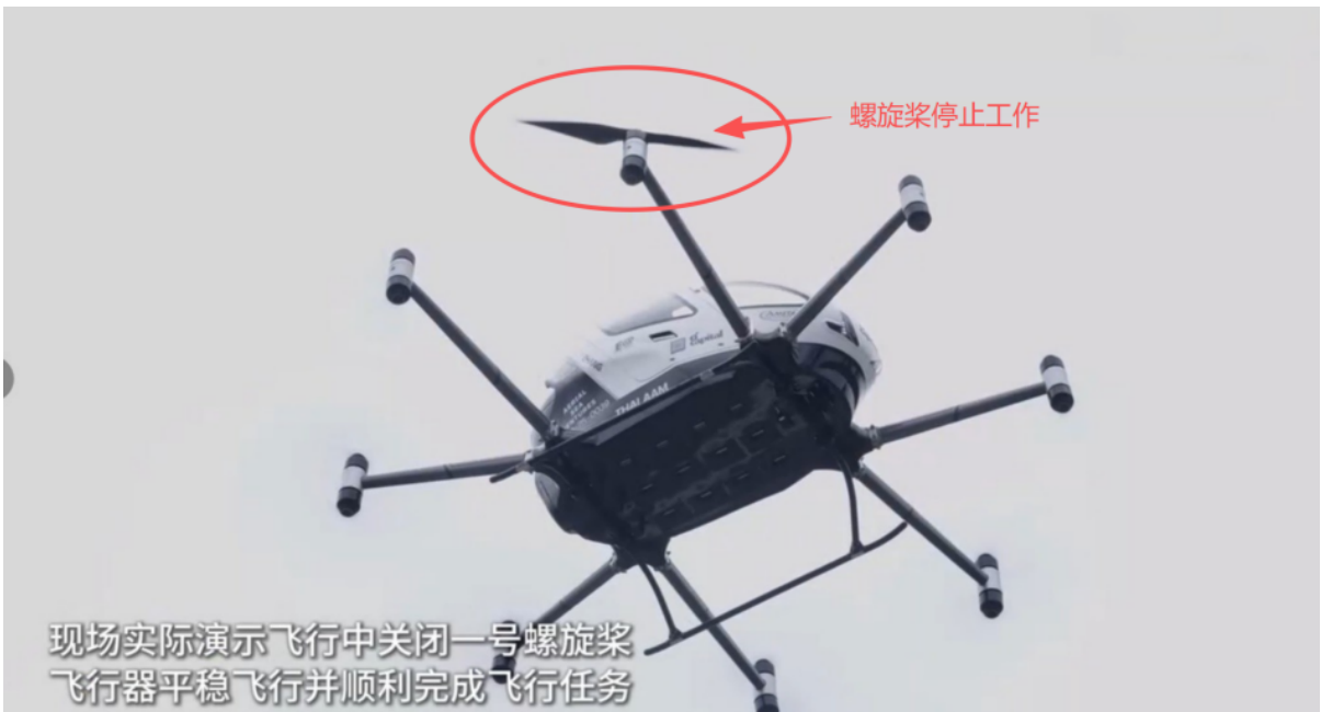
(Image: EH216-S demonstrated stable flight with a rotor stopped in Thailand)
