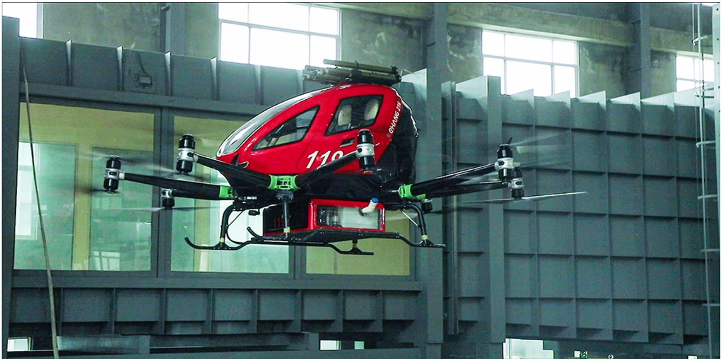
*(Picture: EH216F undergoing the wind resistance test)*
