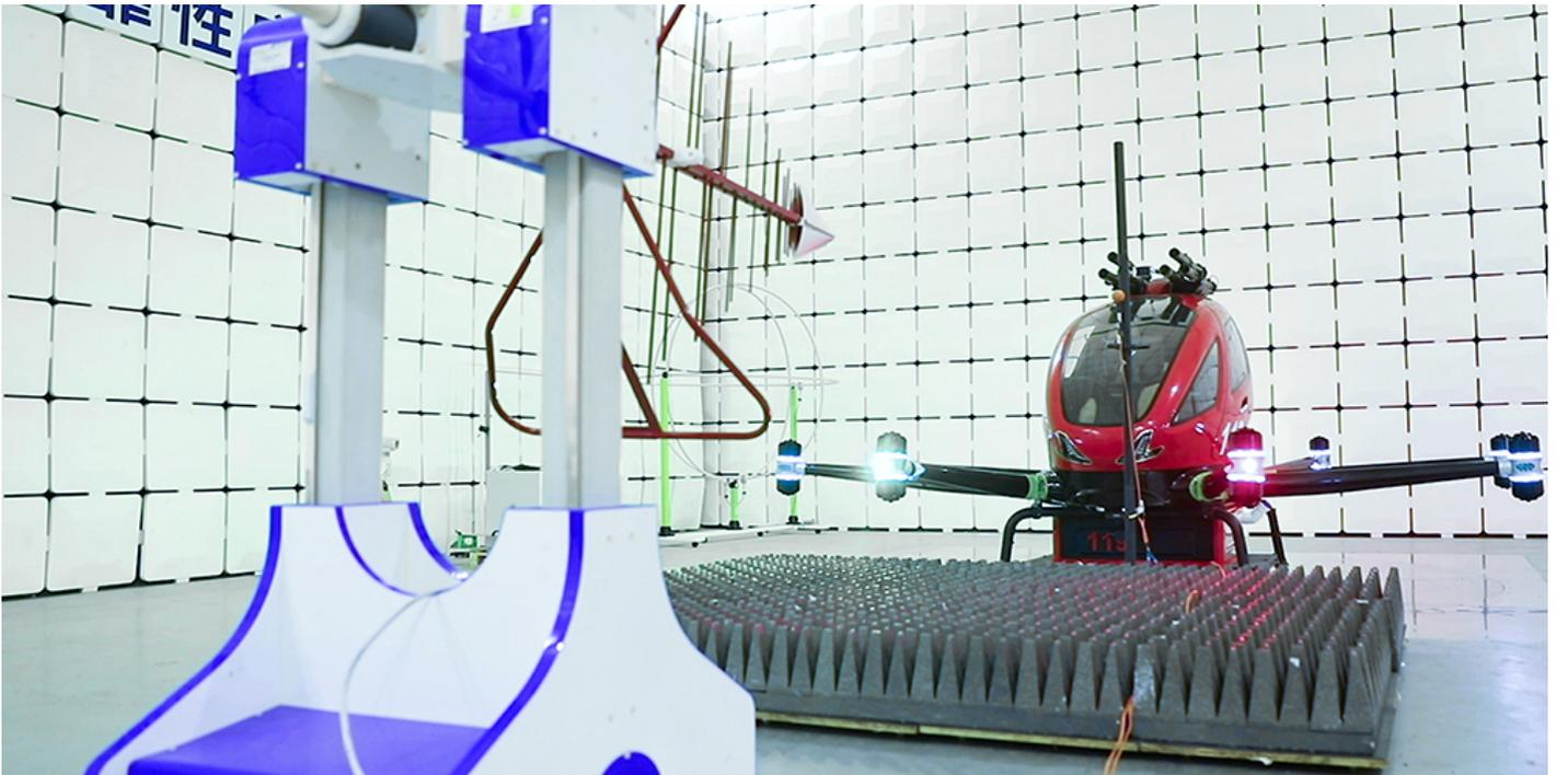
*(Picture: EH216F undergoing the electromagnetic compatibility test)*
