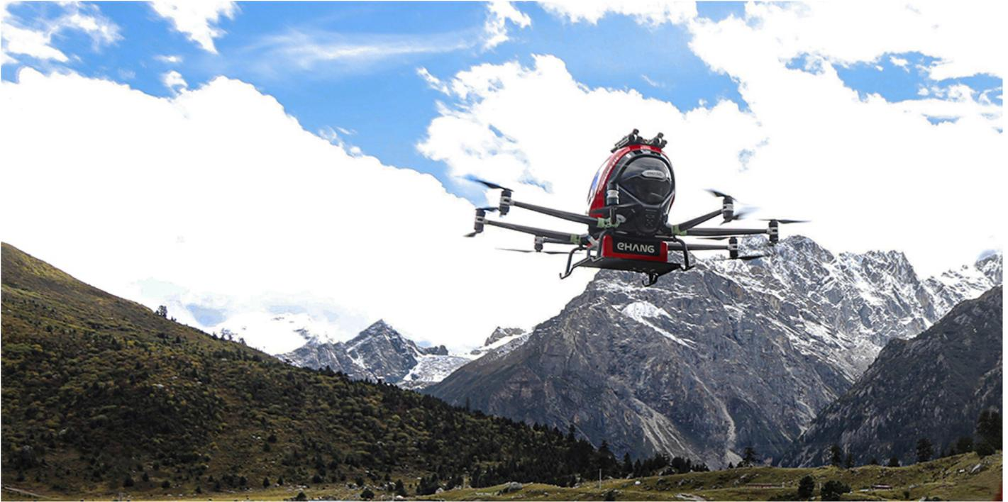
*(Picture: EH216F undergoing the high-altitude flight test at 3,200 meters above sea level)*
